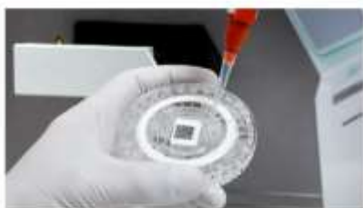
Take the blood sample and insert the sample material of choice (serum, plasma or whole blood) into the rotor of choice.
